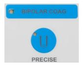
In the "Bipolar COAG" operator panel identified in blue on the right of the front plate, a lamp (8) indicates activation of the bipolar coagulation current. One current type is available for bipolar coagulation:
