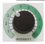
The output adjuster (7) is used to set the output power. The output setting ranges from a specified minimum value up to a maximum value depending on the selected current type (see technical data, chapter 9.1). Here the increase in the output power is close to linear with the rotation angle. See the diagrams below for the relationship for each current type.
