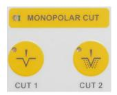
In the "Monopolar CUT" operator panel identified in yellow on the front plate, a lamp (2) indicates the activation of the cutting current and two different current types are available for cutting:
